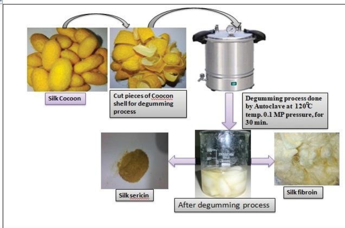
Figure 3: Schematic diagram of extraction process of sericin from silk cocoons (Adopted from Saha et al. , 2019).
