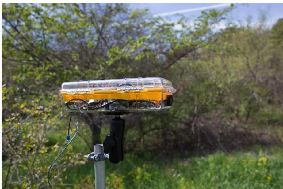
Active infrared camera trap for detecting wildlife
