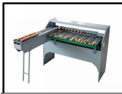
Fig 10: Egg Sorting Machine
