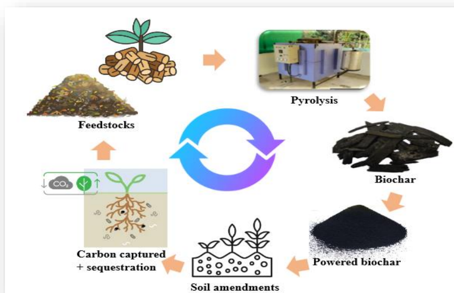
Fig. 1 Systematic representation of synthesis and application of biochar
